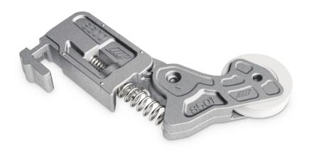
Corner joint for screen doors, casement windows and sliding profiles with square cut. Pre-installation by insertion, tighten and adjustment by Recex® screws. Sold individually or along with ball bearing POM wheel roller. **Montix anti-corrosion coating available on demand.**
